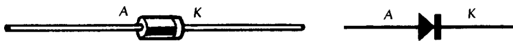
A typical diode with a band at one end to indicate the cathode (K).
